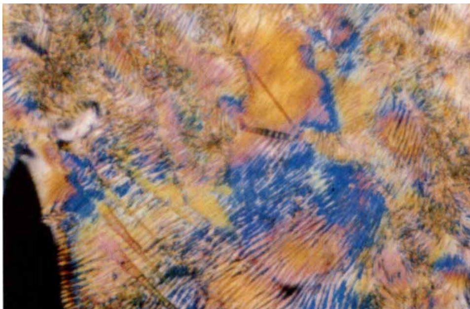
Figure 5. Typical texture in the polarizing microscope of polyesters with cross-shaped mesogens after annealing in the liquid-crystalline phase.
